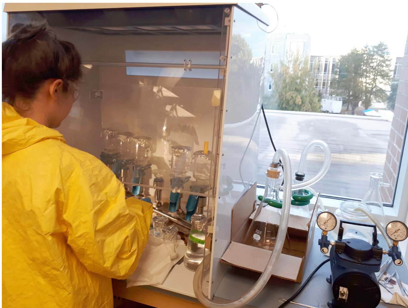
Photo 4. A researcher uses a vacuum pump and filter assembly to filter down tissue samples that have undergone digestion to isolate potential microplastics. We then viewed the filters on a compound microscope and picked off any potential microplastics and placed them onto double-sided tape for spectroscopic analysis. Photo credit: Garth Covernton.
