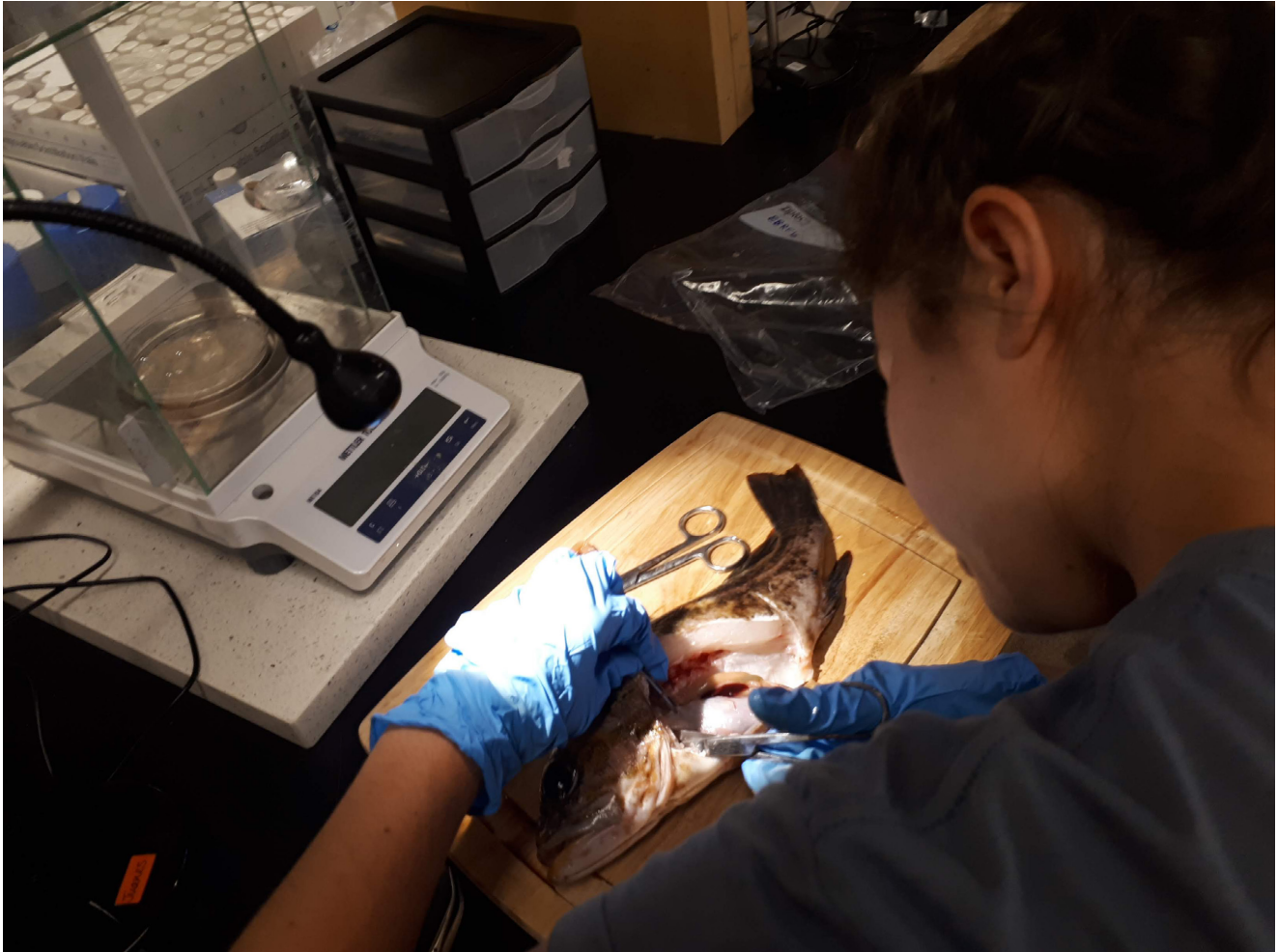
Photo 3. A member of our team dissects a rockfish to remove the digestive tract and liver for microplastic analysis. To isolate microplastics from all animals, we used a potassium hydroxide solution to remove tissues and a sodium iodide solution for sandy samples to float out the plastics from the sand. Photo credit: Garth Covernton.
