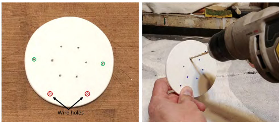
Fig. 20. Drilling of the holes on the discs.
