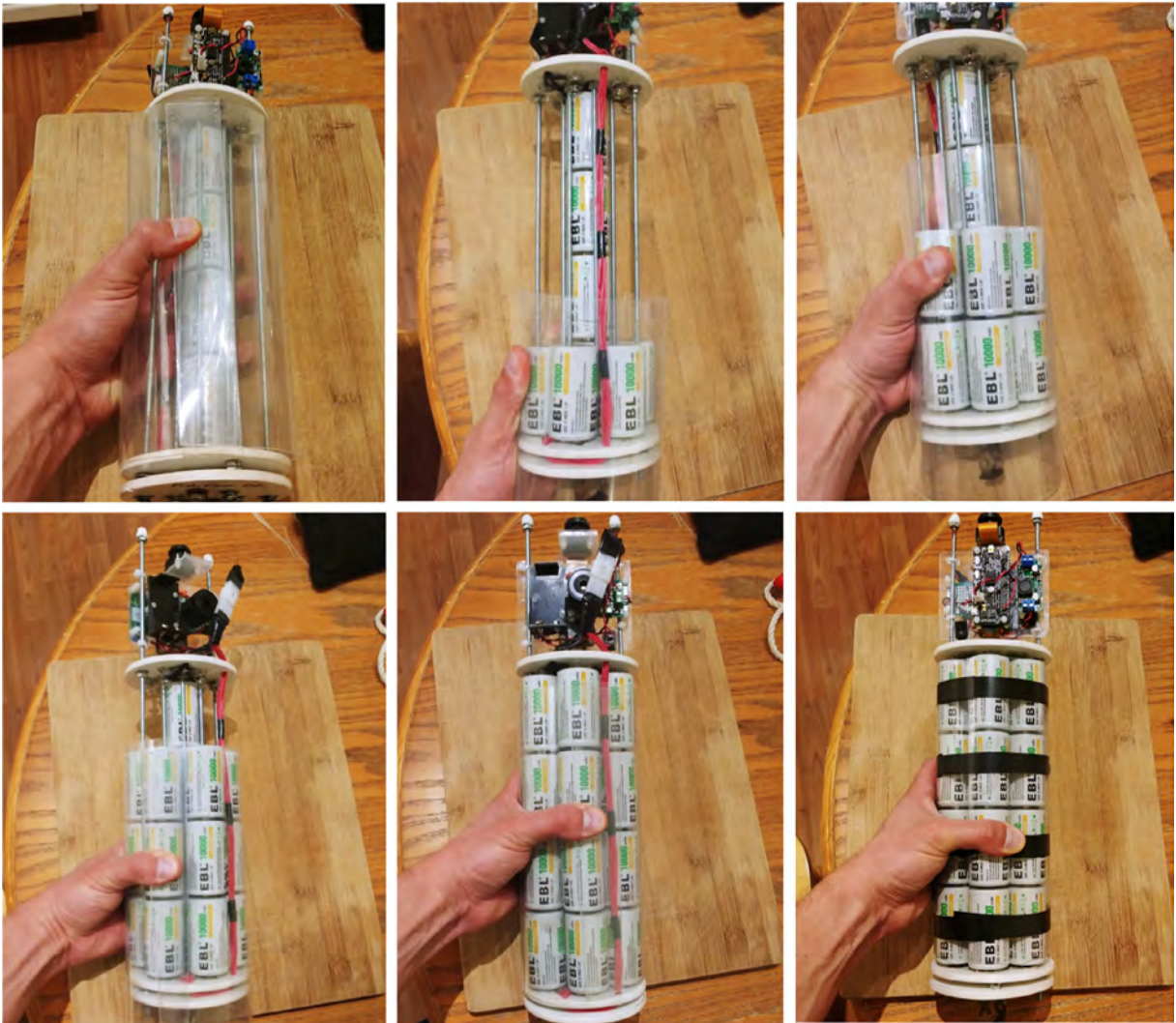
Fig. 36. Installation of the rest of the D-cell batteries.
