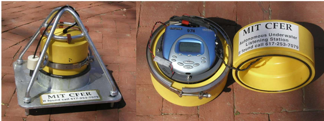
Figure 2. Automatic Listening Station (AULS) used to record haddock sounds in the Gulf of Maine during 2003-2004 and 2006-2007. Left: Complete AULS in protective steel mount ready for deployment. Right: Nomad recorder shown inside housing prior to sealing.
